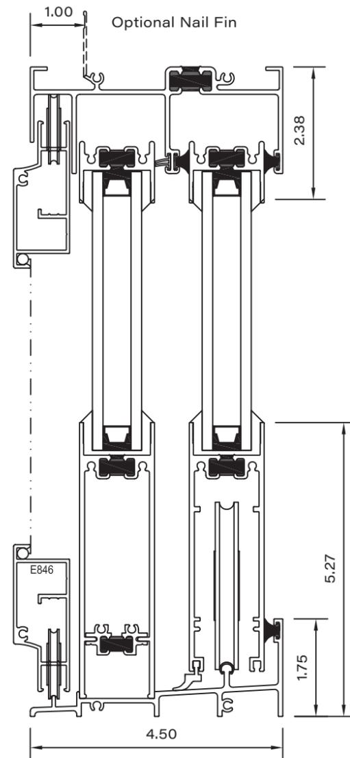
vertical section with 3.00" diameter rollers and 1.75" threshold
