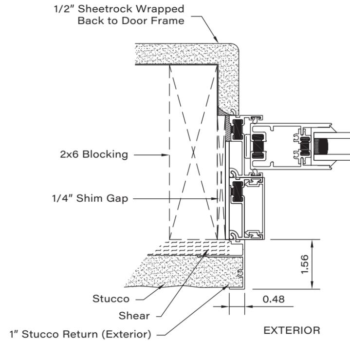
1" stucco return wall construction profile @ stud multi-slide stacking door jamb application
