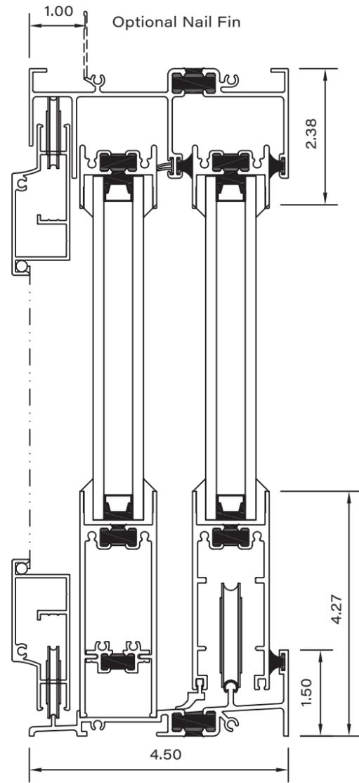
vertical section with 1.81" diameter rollers and 1.50" threshold
