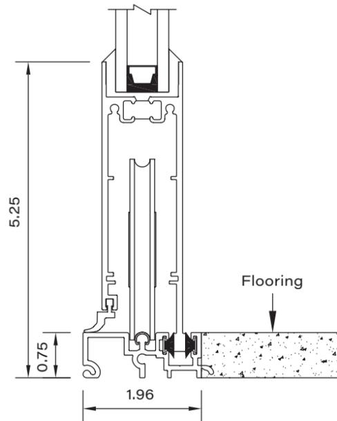
flush threshold with 3.00" diameter roller
