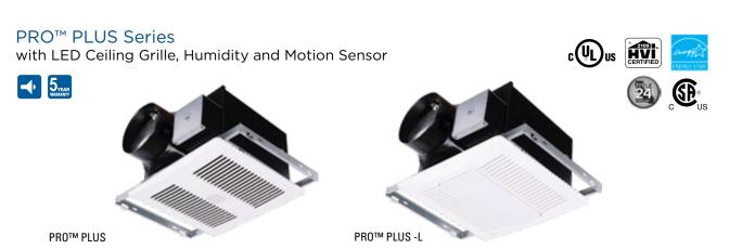
User-adjustable 80/90/110/140 cfm fan with a ceiling grille, backdraft damper, humidity and motion sensor. The fan provides 4 different airflows: 80-90-110-140 cfm. Uses a 6" metal duct. The product is provided with an adjustable 12-24" EZ bracket for ease of installation. This model holds an ETL listing and conforms to UL and CSA safety standards. ENERGY STAR® and HVI qualified, California Title 24 Listed.
